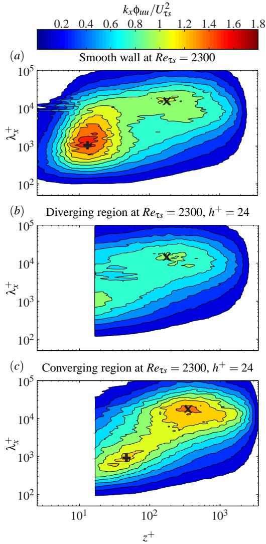
Figure 5: Contours of pre-multiplied streamwise energy spectra for the smooth wall case (a) and above the diverging (b) and converging (c) regions at  $Re_{\tau_s} = 2300$ .
