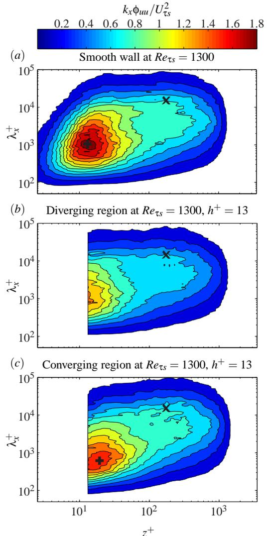
Figure 4: Contours of pre-multiplied streamwise energy spectra  $k_x \phi_{uu} / U_{\tau_s}^2$ , where  $k_x$  is streamwise wavenumber and  $\phi_{uu}$  is the energy spectra of streamwise velocity fluctuations. The pre-multiplied spectra is plotted as a function of wall-normal position  $z^+$  and energetic streamwise length-scale  $\lambda_x^+$ . Plots are shown for the smooth wall case (a) and above the diverging (b) and converging (c) regions at  $Re_{\tau_s} = 1300$
