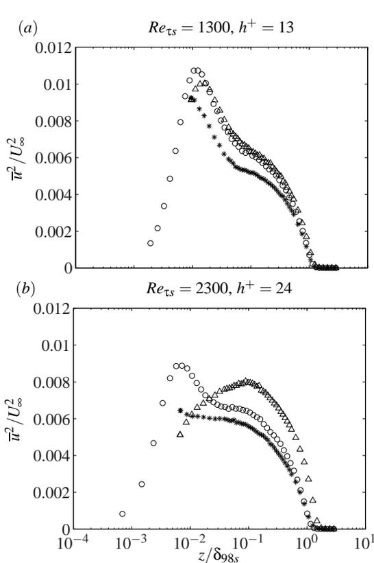
Figure 3: Turbulence Intensity for  $Re_{\tau_s} = 1300$  (a) and  $Re_{\tau_s} = 2300$  (b) over the diverging (\*) and converging ( $\Delta$ ) regions of the rough surface, and for the smooth wall case (o). Turbulence intensity is non-dimensionalised using free stream velocity  $U_\infty$  and distance from wall is non-dimensionalised using boundary layer thickness over the smooth wall  $\delta_{98s}$
