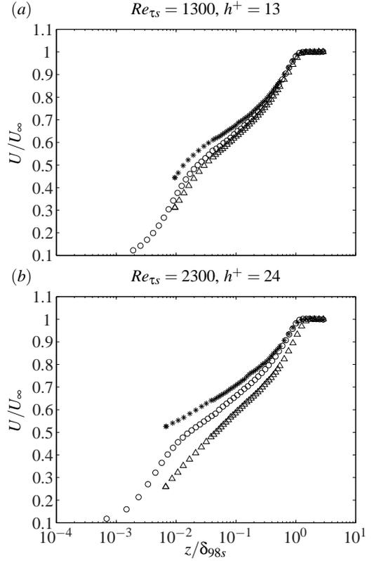
Figure 2: Mean velocity profile for  $Re_{\tau_s} = 1300$  (a) and  $Re_{\tau_s} = 2300$  (b) over the diverging (\*) and converging ( $\Delta$ ) regions of the rough surface, and for the smooth wall case ( $\circ$ ). Velocity is non-dimensionalised using free stream velocity  $U_\infty$  and distance from wall is non-dimensionalised using boundary layer thickness over the smooth wall  $\delta_{98s}$ .
