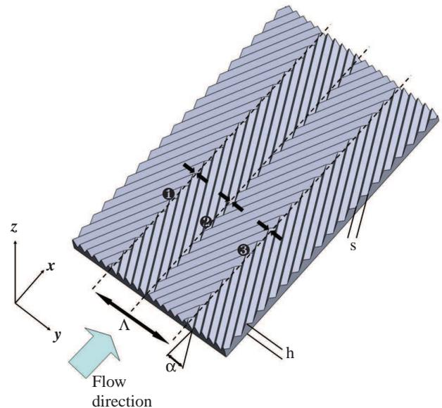
Figure 1: Schematic diagram of converging / diverging riblet pattern, showing regions of converging (regions ① and ③) and diverging (region ②) spanwise flow.
